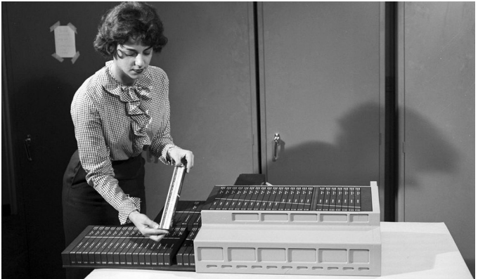
Technician assembling the micrologic and core memory panels that make up the Apollo Guidance Computer into their housing.
