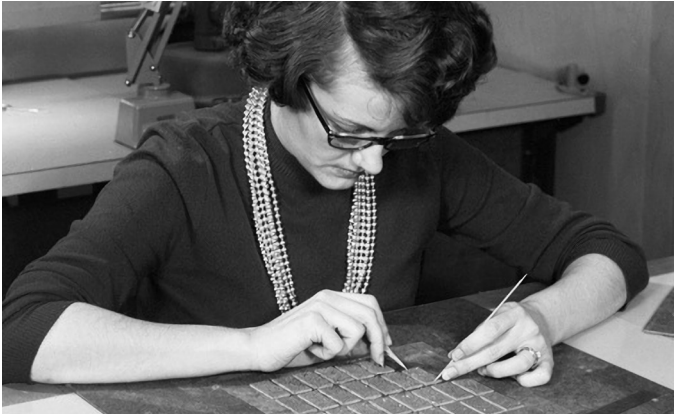
Engineer stringing the sense inhibit wiring components of the Apollo Guidance Computer erasable memory.
